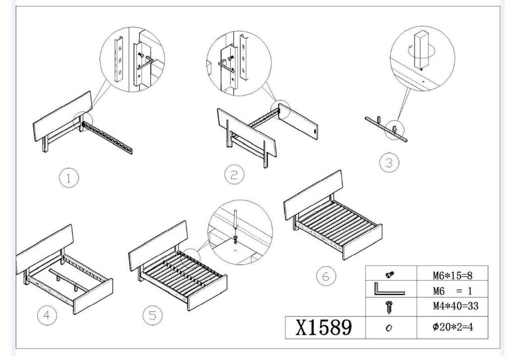
\*\*\*Step 5 – Slats have 3 screws to attach them to the side rails & centre support rail.
